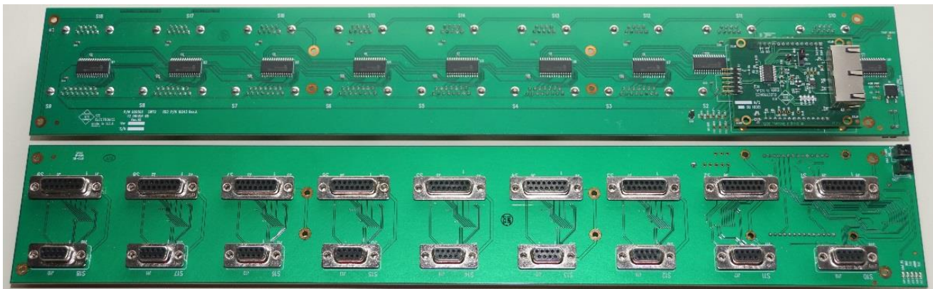
A 72-Channel Switch Driver Board. The component side (top) shows the expander chips and the I 2 C01 Module on the right. The connector side (bottom) shows the switch mating connectors.
