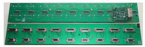
Some OEMs have built backplane boards to handle decoding, interconnections and interfacing using ribbon cables to connect to the interface board. However there are reliability issues with ribbon cables, especially in military or other high-reliability systems. The Modular System Controls approach is to use distributed processing. A small module about the size of a credit card containing a low cost
